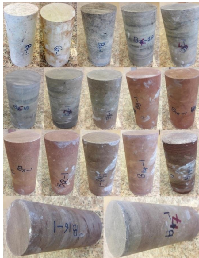
Figure 2: Prepared samples for compressive strength. (by researchers)
